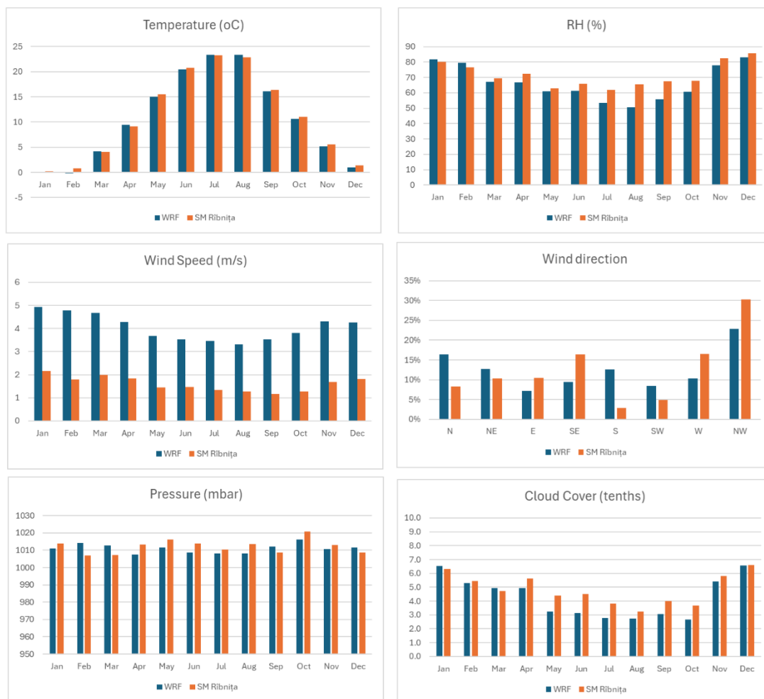
Figure 2.3: Comparison of the monthly values of the main meteorological parameters based on measurements at Rîbnița station and the results of the WRF prognostic model at the location of the cement plant. Data covers period 01/01.2021-31/12/2023.
